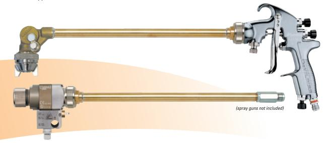
The DeVilbiss extension range is manufactured from brass with stainless steel needles as standard, they are available for Advance *HD* manual and Cobra 2 automatic pressure spray guns. When ordering ensure the part number for the model is completed with the required length in inches. Other lengths and flexible extensions are available upon request.
